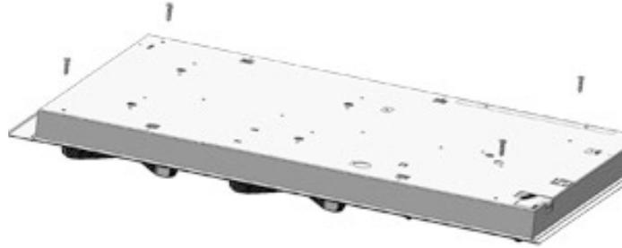
**Attention.** Do not use electric screwdrivers or torque wrenches to fix the top. Hand tighten without forcing the screws.
